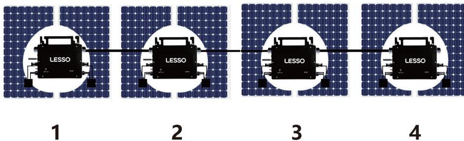
1. LSMT800TL-H1 @Single-Phase 230V grid Maximum 4 units LSMT800TL-H1 micro PV inverter per branch.
