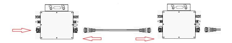
\*Note: The length of AC cable on microinverter is roughly 1m, if the distance between two microinverters is more than 1m, please use an AC extension cable between two microinverters.
