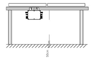
required to ensure the communication quality between the WIFI and the microinverters.
