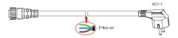
\*Note: Using the AC grid-connected cable, it can be plugged directly into the socket Fast grid connection for use, the maximum number of machines with 3 sets;
