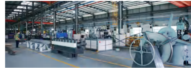
○ U-channel steel production line
