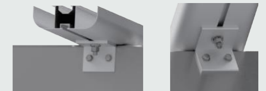
Installation Node Diagram of Waterproof Guide Rail and Cross-Beam:
